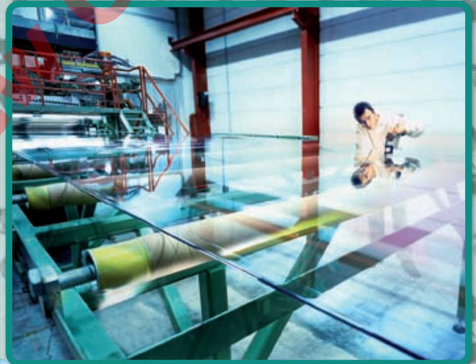
This extruder shapes plastic pellets into sunroofs.
